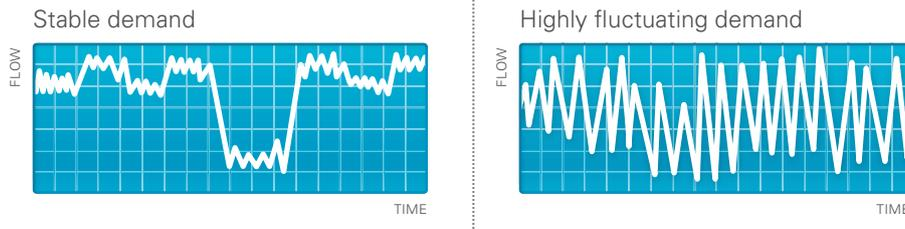
The ZH 350+ handles air demand fluctuations more effectively than turbo technology could do up to now. Its fast transitions between load and unload operation eliminate the need for expensive blow-down of compressed air in times of low air demand.
